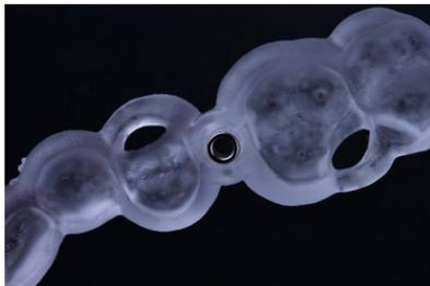
Image 4 - Intaglio surface of a Luxa Print Ortho 3D printed surgical guide with ideal adaptation to the metal sleeve.
