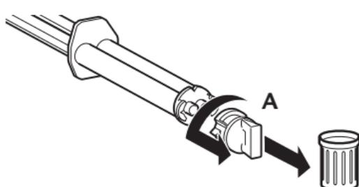
1. Before attaching the mixing tip, remove the cap [A] or used mixing tip after twisting it 90° counterclockwise, and discard it.
