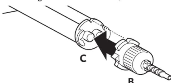
2. Attach a new mixing tip [B].
