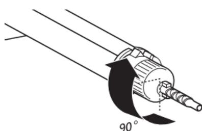
3. Turn the mixing tip clockwise 90° to lock it into place.
